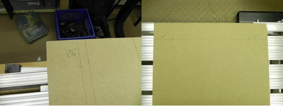
Mark holes for hold down/spring bolts at rear edge of seat. These holes are app 1 ¾" from edge on the 4" line marked earlier. These holes will be app 2" from sides of seat when viewed from the top
