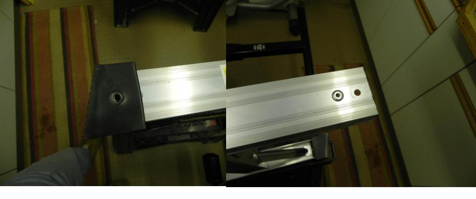
Reinstall foot removed earlier and use as guide to drill new mounting hole. Remove foot, drill hole, reinstall foot and rivet in place.
