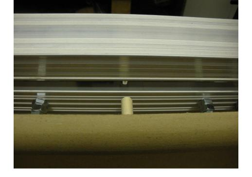
Cut dowel to size and dry fit in mounting hole. Make sure dowel does not over travel switch when seat is fully traveled down. Adjust by sanding or filing and then glue in place.
