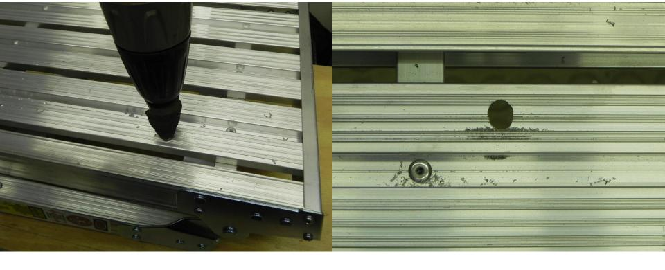
Drill holes for hold down bolts to pass through. These holes will need to be oversized and oval to allow bolt to pass through. I used a file to lengthen them fore/aft until the bolt would swing through and have clearance
