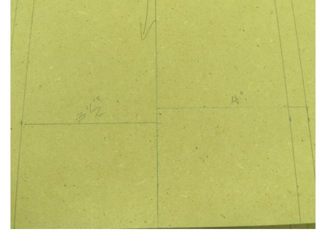
Cut seats app 12" X 12". Mark the centerline of the seat and then two line 2 3 ½" and 4" on either side of the centerline. The 3 ½" line will be the center of the hinge and the 4" line will be the mounting bolt location. (these are the dimensions I used you can adjust as necessary based on hinge type/size.
