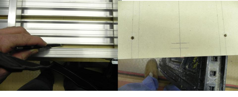
The switch will be activated with a dowel mounted in the seat passing through this space. Using the bench as a guide mark both sides of the gap on the centerline of the seat.
