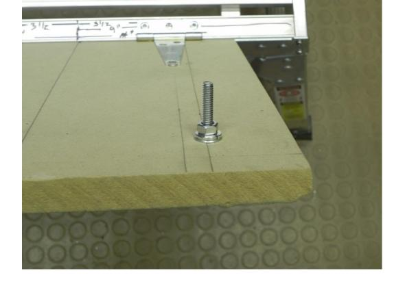
Attach carriage bolt to seat using flat washer and lock washer
