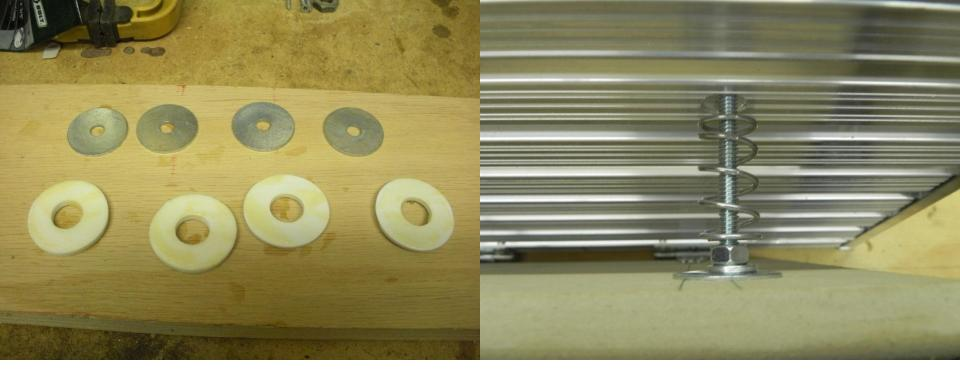
Add springs to the carriage bolts and pass through the holes in the bench. Secure on the backside using fender washer and nylon locknut. The washers will 'bang' on the backside of the bench so I glued foam washers to the fender washers. Felt, foam or other cushioning material can also be used.
