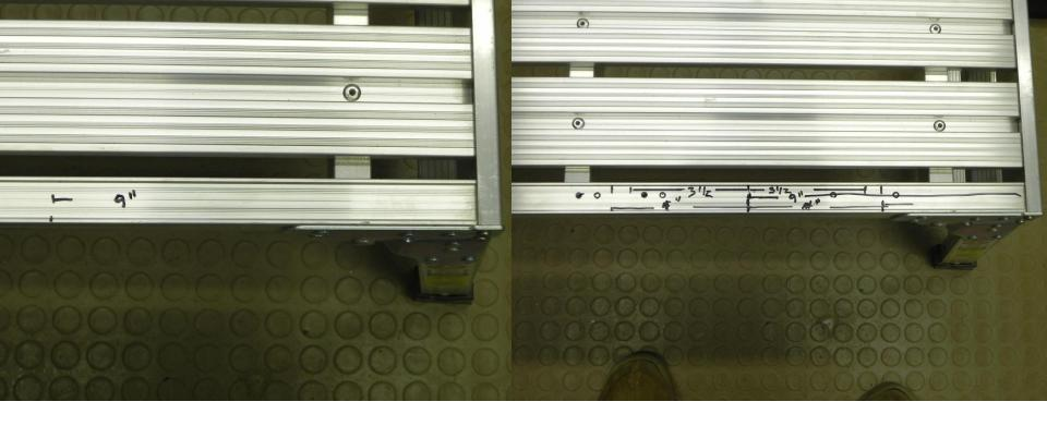
Mark centerline of seat 9" from edge of bench. Use seat with hinges attached. Align centerlines and mark mounting locations for hinges on bench. Drill holes in bench and attach hinges. (I used rivets to attach hinges. It was easier to remove hinges from seat, rivet them them to the bench and then reattach the seats.
