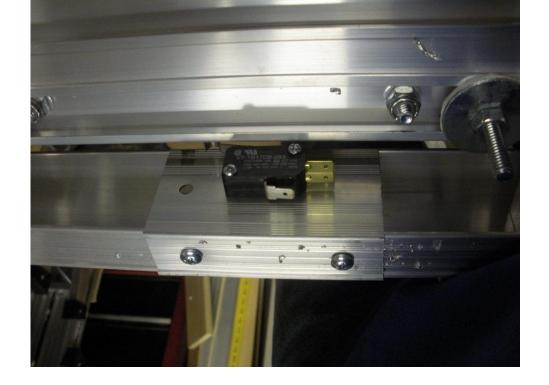
Tighten hold down/spring bolt bring seat down until dowel is just in contact with switch. Make sure switch is not overtraveled when seat is fully down.
