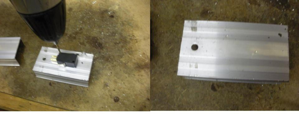
Use excess leg removed earlier for switch mounting. Place switch on leg and mark hole mounting locations. Drill holes and attach switch – rivet or small bolt/nut.
