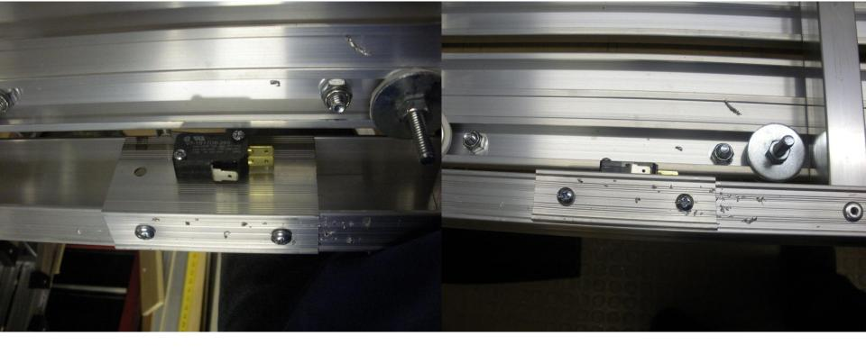
Attach leg piece with switch to bench making sure to align switch contact with hole in seat. I used self drilling screws to make repair easier later
