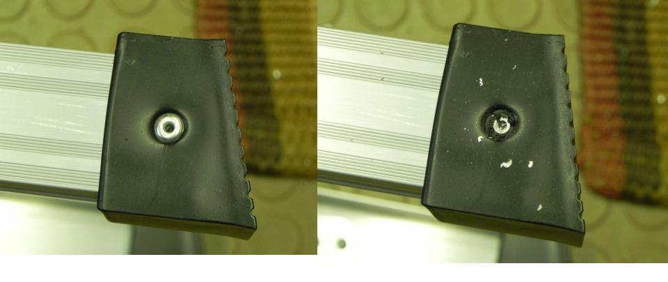
The rubber feet need to be removed. Drill out the head of the rivet and remove foot. You may need to pry a little around rivet.
