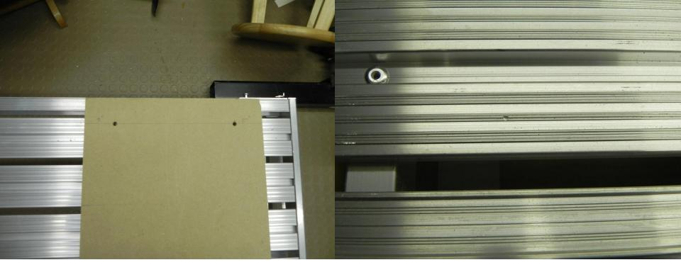
With seat attached to the bench use the 2 holes drilled in the seat to mark hole locations on the bench
