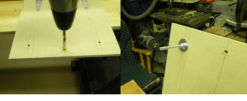
Drill a hole ½" deep taking care not to drill all the way through. A dowel will be glued in this hole later to activate switch.
